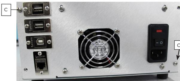
5. Slide the power supply and controls assembly out of the base assembly.
